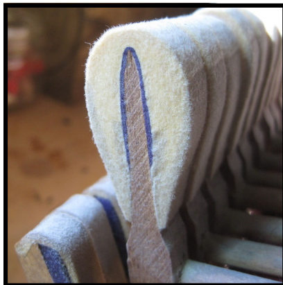
Worn hammer after filing
