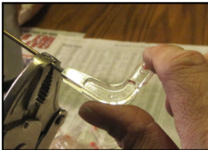
New plastic elbows being installed in a spinet.
