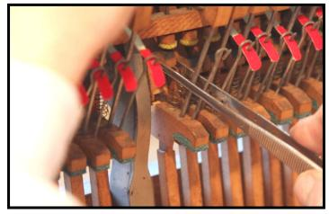
Special 8'long tweezers used to position parts.
