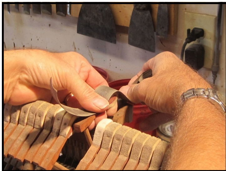
Hammers being filed to remove cut marks.
