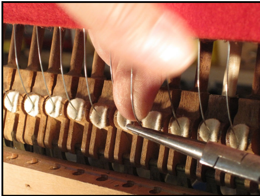
A new set of original-type springs being given final adjustments in the action.
