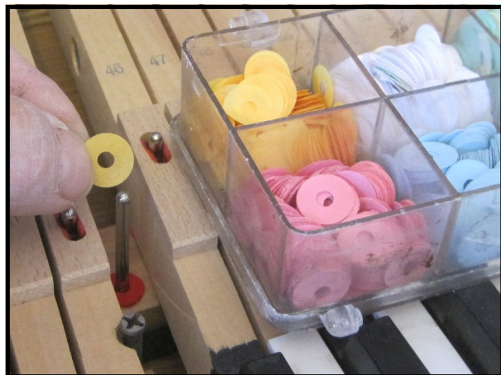
.002"paper punching being installed
