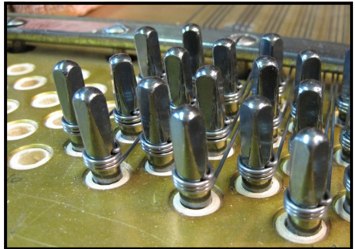
New tuning pins and strings being installed.
