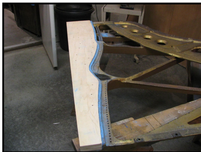
Underside of cast iron plate with new pinblock installed.
