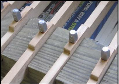
After the keys have been returned to the piano they will be given a final test for fit and will be eased (adjusted) if necessary for an absolute consistent feel from one note to the next. If your piano action is in good regulation and the hammers are in good shape, your piano should be as responsive to your touch as the day it left the factory and will be a pleasure to play once again.
