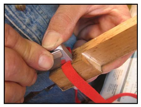
After the felt is inserted into the key, a sizing caul (a precision fitting device) is used to hold the felt in place while a razor is used to slice it precisely to the correct length.
