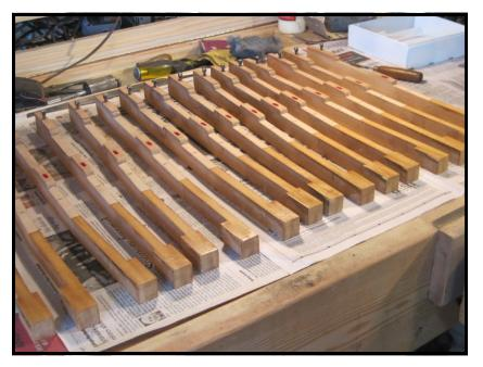
The new tops are glued to the keysticks with a special adhesive which produces a rock solid bond between the keytop material and the wooden keystick. This type of glue creates a bond stronger than the wood itself.
