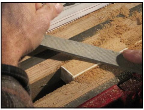
ing files to produce an edge which is perfectly flush to the wooden keystick. When done correctly, there will be no overhanging edge along the sides of the keys.
