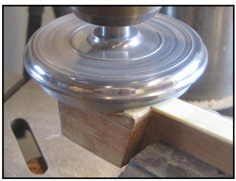
to compensate for the greater thickness of the new keytop material. This milling down process gives a completely flat surface on which to glue the new keytops.
