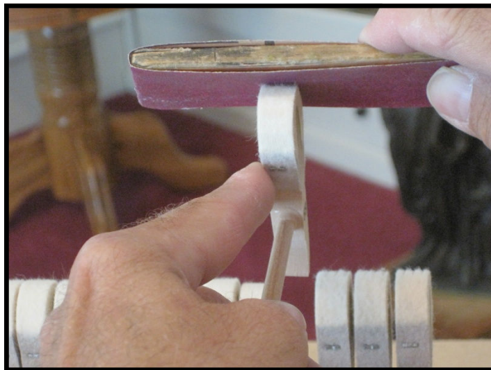
Hammers being filed to remove cut marks.
